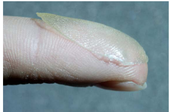
Fig. 2. Illustration of a fake made of latex, produced from Siligum mould using the direct method.
