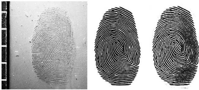
Fig. 1. Illustration of a deposited fingerprint (left), the final image (middle) obtained after processing it using Adobe Photoshop® CS2 (including manual correction of artifacts), and a capture (right) obtained from the final fake fingerprint elaborated with glue from the indirect cast printed on an acetate sheet.
